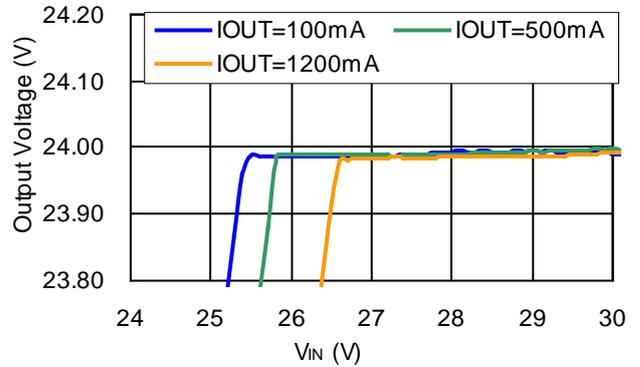
30) Input voltage vs. Output voltage (Version C/D)
