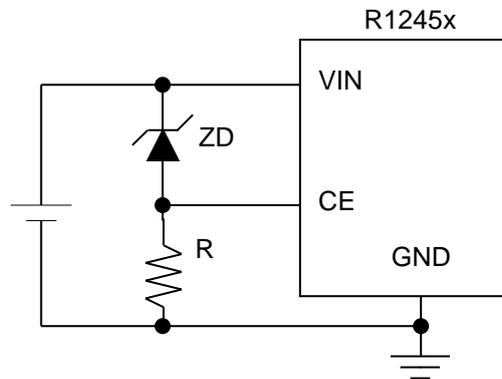
**Figure 9. Low input voltage countermeasure circuit with using ZD**
