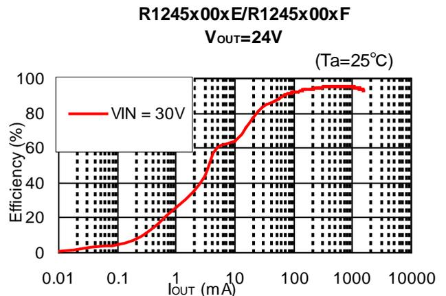
24) Output current vs. Efficiency (Version G/H)
