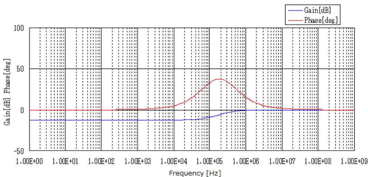
Figure 3. Transfer function BODE plot from  $V_{OUT}$  to FB (R1=3.75k $\Omega$ , R2=1.2k $\Omega$ , Cspd=470pF)
