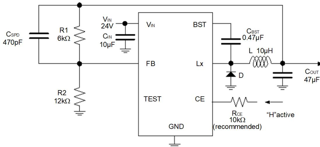
R1245x00xA/B Typical Application Circuit, 330 kHz,  $V_{OUT} = 1.2\text{ V}$ ,  $V_{IN} = 24\text{ V}$
