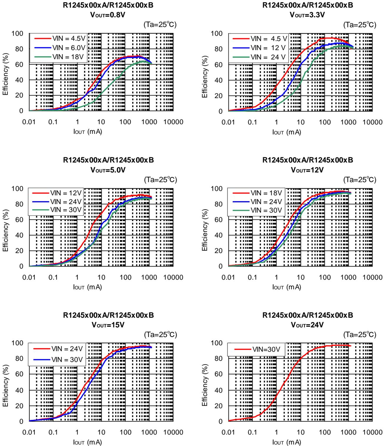
22) Output Current vs. Efficiency (Version C/D)
